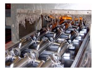
The **disadvantages** of furnace brazing have to do mainly with furnace issues, e.g., the cost of equipment (versus flame brazing), higher power consumption, and furnace maintenance requirements. In addition, somewhat more attention has to be paid to **joint design** because the brazing takes place in the furnace chamber, and is not easily
